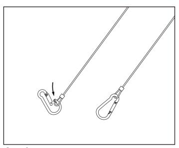
Step 6 Clasp the hook through the aircraft cable loophole created.
