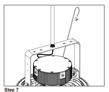
Clasp the hook onto the allocated bolt on the fixture mount.
